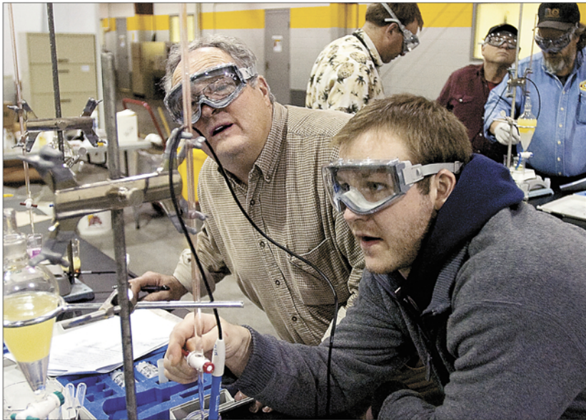
Eric Collar of Eaton Rapids, left, checks levels of potassium hydroxide as Ryan Fitzgerald of Saginaw carefully drops some into a solution to determine its acidity during an advanced biodiesel class Wednesday at Michigan Brewing Company in Webberville, Mich. The class is three days long, starting with a beginning biodiesel class and ending with a production class in which students make a large batch of biodiesel. Collar said he would like to be able to make his own fuel — he drives a truck that can use biodiesel.
